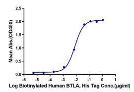
Immobilized Anti-BTLA Antibody, hFc Tag at  $0.5\mu g/ml$  (100 $\mu$ l/well) on the plate. Dose response curve for Biotinylated Human BTLA, His Tag with the EC50 of 8.0ng/ml determined by ELISA.
