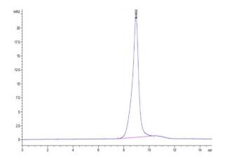
The purity of Biotinylated Human BTLA is greater than 95% as determined by SEC-HPLC
